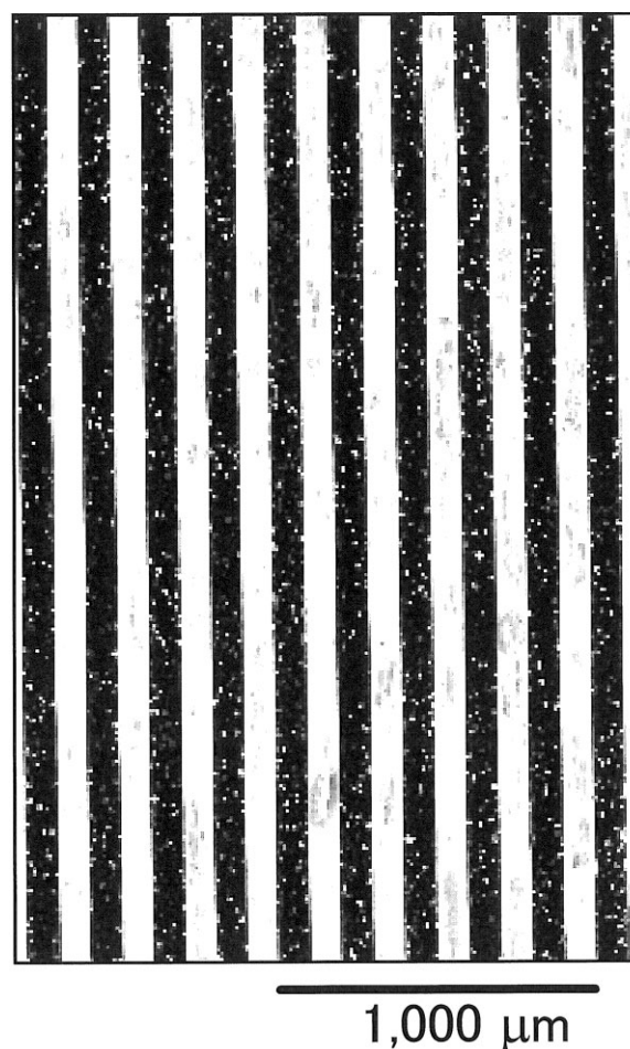
Figure 6 Fluorescence micrograph illustrating how FITC could be templated onto hydrophilic/hydrophobic patterned glass substrates. The hydrophilic/hydrophobic patterned surface was prepared with a photomask with a 100/100 μm line/space width. The bar on the lower right indicates 1000 μm.
